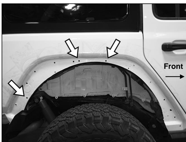
(Fig 3) Fender Liner will attach to the (3) factory locations typically used to attach aftermarket fenders (arrows). Use either the hardware supplied with the fenders (must be 6mm hardware) or the included 6mm Combo Bolts to attach the Fender Liner to these mounting points (passenger/right side pictured without fender for instruction purposes only)
